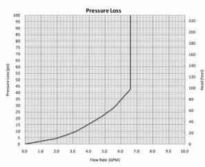
Maximum flow rate is limited to 6.6 GPM.
