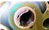
Scale buildup from untreated water.
