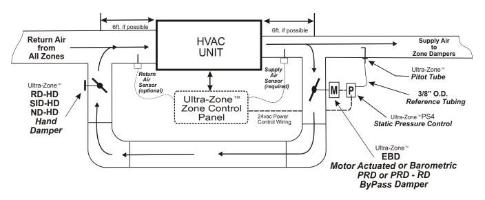
Note: This drawing of the Bypass damper, Hand Damper, Static Pressure control and Related duct work is intended to serve only as a guide. Your actual duct work layout and components may differ. Use the graphic as a guide when planning or designing a Zone system regardless of the Equipment type, Duct layout and Airflow configuration.
