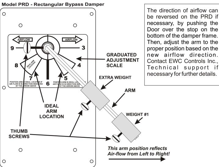
be reversed on the PRD if necessary, by pushing the Door over the stop on the bottom of the damper frame. Then, adjust the arm to the proper position based on the new airflow direction. Contact EWC Controls Inc., Technical support if necessary for further details.
