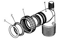
V3007 1" PVC Male NPT Elbow Assembly Standard
