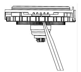
The drive cap assembly contains the drive cap, the main drive gear, drive cap spline, piston rod and various other parts that should not be disassembled in the field. The only replaceable part on the drive cap assembly is the o-ring. Attached to the drive cap assembly is the main piston and, if a regenerant is used, a regenerant piston.
