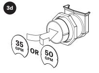
Depending on which flow rate is desired, snap-in the "35 GPM" or "50 GPM" white flow control plate as shown on inlet saddle adapter.
