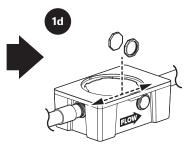
Firmly hand thread test caps onto inlet and outlet diffusers as shown.
