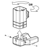
Rotate diffuser top toward desired outlet, while ensuring foot is pointed toward the back wall of the unit. Reattach to foot using set screws.
