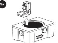
Remove inlet diffuser.
