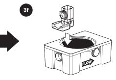
Seat inlet diffuser firmly into saddle adapter.
