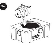
Re-install saddle adapter, ensure flow control plate opening is down as shown.
