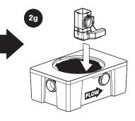
Seat diffuser firmly into saddle
