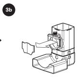
Remove red flow control plate from inlet diffuser and discard.
