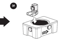
Seat inlet diffuser firmly into saddle adapter.
