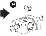
Firmly hand thread test caps onto the unused side outlets.
