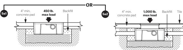
Backfill evenly around tank using crushed aggregate (approximately 3/4" size rock or sand, with no fines), finish with a minimum 4" thick concrete pad. Vent per local code.
