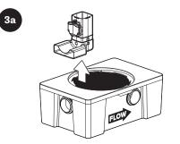
Remove inlet diffuser.
