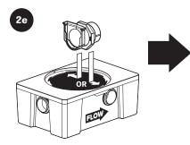
Install saddle adapter on desired outlet.
