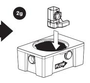
Seat diffuser firmly into saddle
