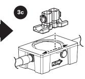
Replace the inlet and outlet diffusers.
