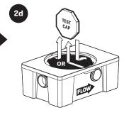
Remove pre-installed test cap from desired outlet and install on straight-through outlet.
