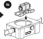
Remove the inlet and outlet diffusers.
