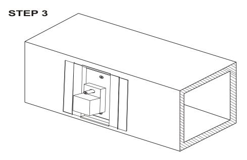
Insert the damper and put in the four corner screws. To secure the damper to the duct board.
