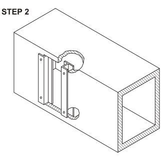
Slide the side brackets over the duct board as shown. Be sure the bracket is positioned so the flanges with the holes are towards the inside of the duct. Be sure to screw the adaptors to the duct with  $1\frac{1}{2}$  " or 2" screws.
