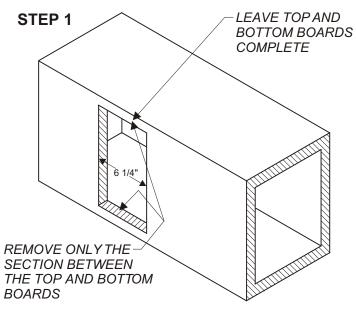
Each kit should contain two identical side brackets. Remove a section of the duct 6 1/4" wide. Cut <u>between</u> the top and bottom boards being sure to leave them in place, including their edge.
