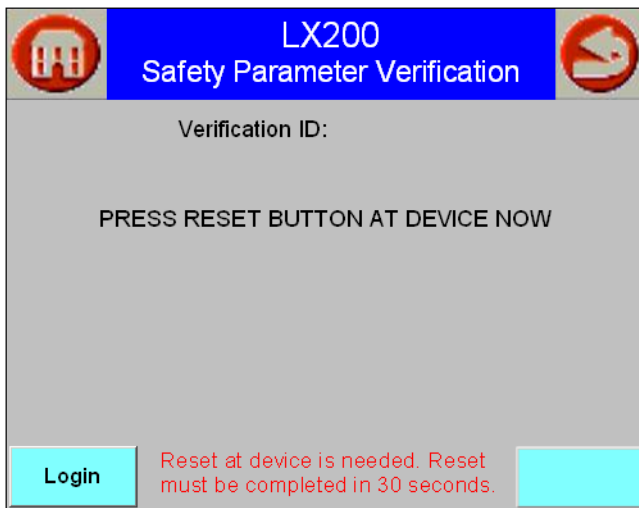
Figure 6: Physical Reset Required
