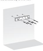
3 Align the grooves on the back of the water heater with the tongues on the mounting bracket and hang the water heater from the bracket.
