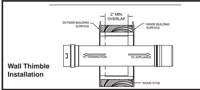
3. Install the Wall Thimble by inserting the larger of the two parts on the appliance (interior) side.
