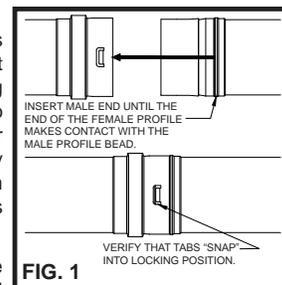
**NOTE:** When assembling Corr/Guard single wall vent, always install the female flue end elevated above the male flue end. The "UP" arrow will point to the elevated female flue end. Change of directions are made by using a male to male or female to female adapter depending on the flow of the condensate.
