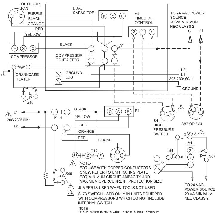
IF ANY WIRE IN THIS APPLIANCE IS REPLACED.IT MUST BE REPLACED WITH WIRE OF LIKE SIZE, RATING, INSULATION THICKNESS, AND TERMINATION.
