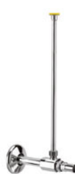
WATER CLOSET SUPPLY 47P1316SD ■ 3/8" IP inlet water closet supply ■ Brass supply nipple ■ Lockshield screwdriver slot angle stops ■ 3/8" OD x 12" flexible riser ■ S/S wall flange
