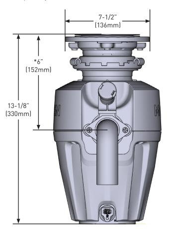
\*NOTE: Distance from bottom of the sink to center line of disposal discharge. Add 1/2" (13mm) when a stainless steel sink is used.
