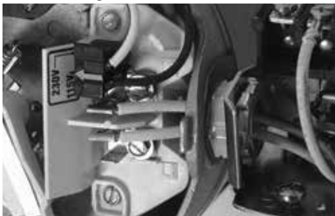
Figure 7 - Voltage set to 115 V, Plug Type
