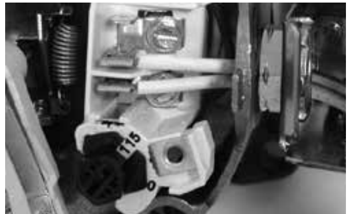
Figure 9 - Voltage set to 115 V, Dial Type
