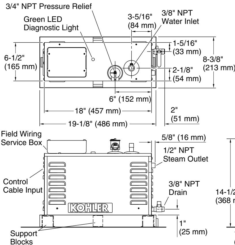
Minimum required access panel is 24" (610 mm) L x 15" (381 mm) H.
