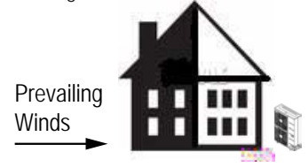
Figure 62: Leeward Side of the Building.
