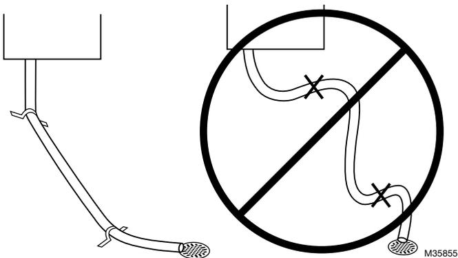
Drain line should have a continuous downward slope to the drain.
