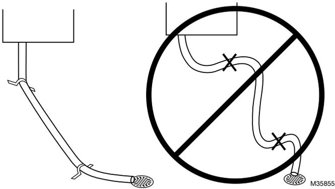
Drain line should have a continuous downward slope to the drain.
