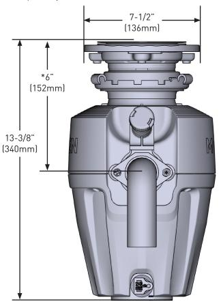
\*NOTE: Distance from bottom of the sink to center line of disposal discharge.
