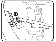
Flip latch back to locked position. Ensure arm does not interfere with fill valve or other parts in the tank.
