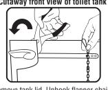
Remove tank lid. Unhook flapper chain from tank lever. Loosen locknut by turning counter-clockwise. (Pliers may be needed) Slide nut off lever arm. Pull lever through tank hole.
