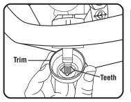
Carefully attach the trim by aligning the teeth at the end of the lever mount with the slots on the trim.
