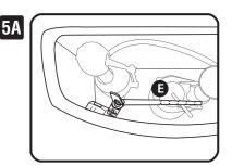
Position the arm parallel to the front wall of the tank, with end of arm directly above flapper.
