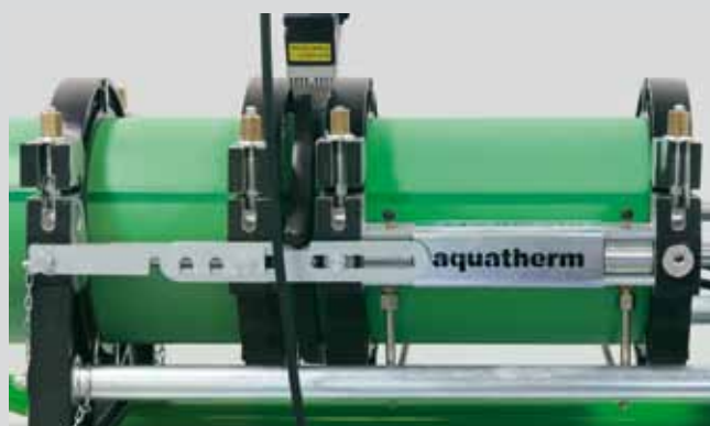
Positioning of heating element
