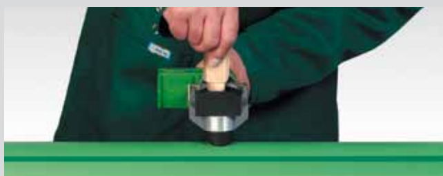
The welding tool is inserted into the pipe wall ...
