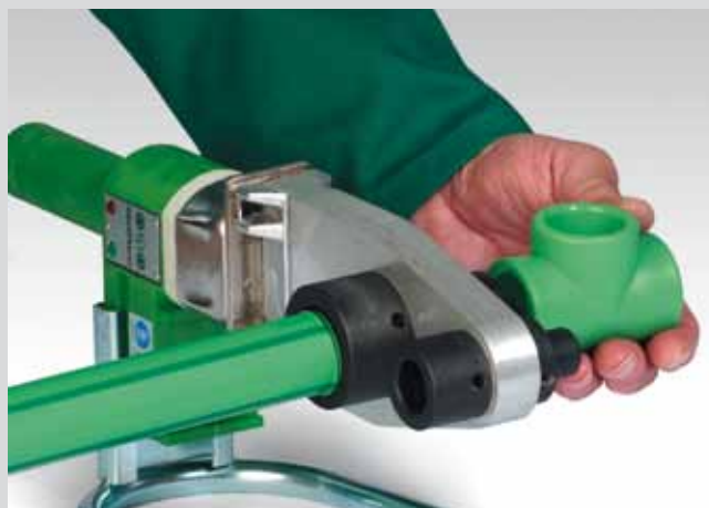
Heating-up of pipe and fitting
