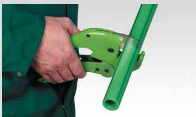
Cutting of the pipe
