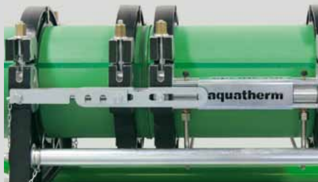
Join the pipes, cool down under pressure
