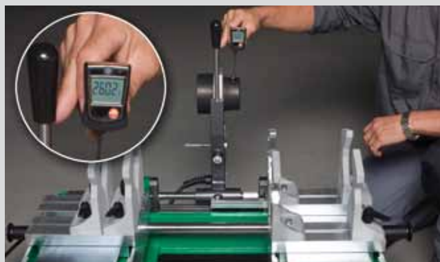
Measurement of temperature at the aquatherm welding machine
