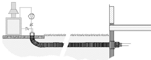
Figure 3-2: Reduce Below-grade Connections
