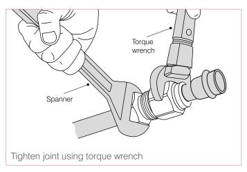
Fully tighten using spanner and torque wrench to the torque values set out in table 8. **Do not over tighten.**
