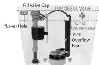
\*The top of the overflow pipe must be a minimum of 1" below tank lever hole.
