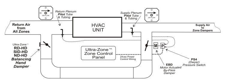
Note: This drawing of the bypass damper static pressure control and related duct work is intended to serve as a guide. Your actual duct configuration may differ and that's OK, so long as all components are installed correctly.
