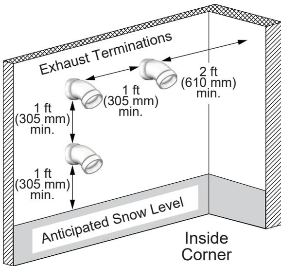
Figure 23 - Multiple Sidewall Terminations
