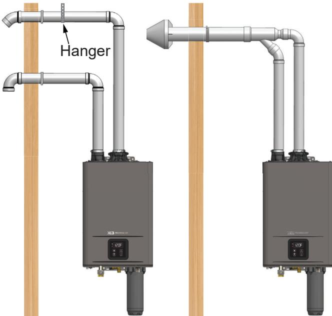
Figure 19 - Power Direct Vent Horizontal Installation
