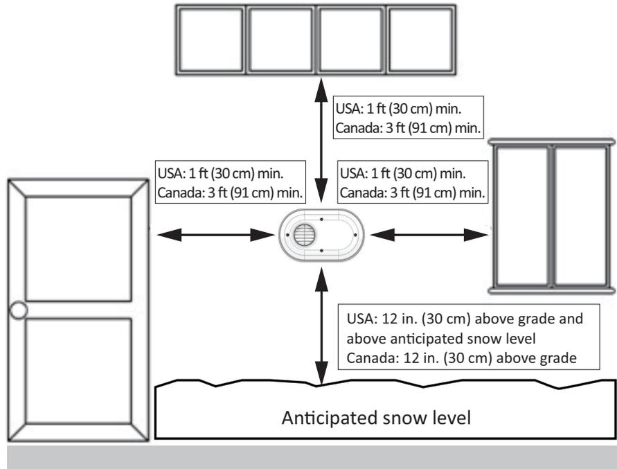
Figure 2 - Minimum Vent Clearance (Indoor Direct Venting)
