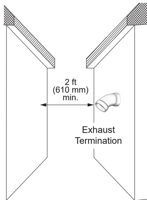
Figure 24 - Sidewall Termination Minimum Distance to Opposite Surface/Wall
