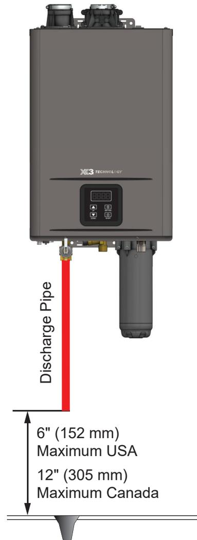
Figure 38 - Discharge Pipe Clearance
