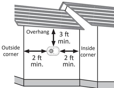
Figure 1 - Overhang and Inside Corner Restrictions
