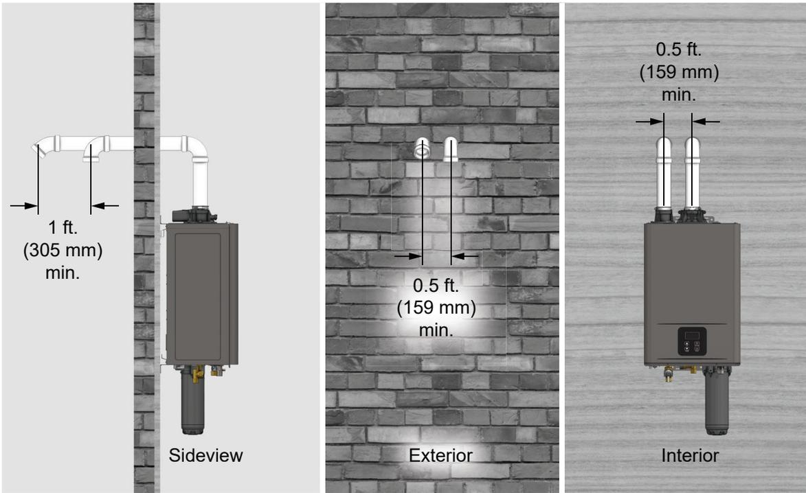
Figure 27 - Separate Sidewall Penetration Example B
