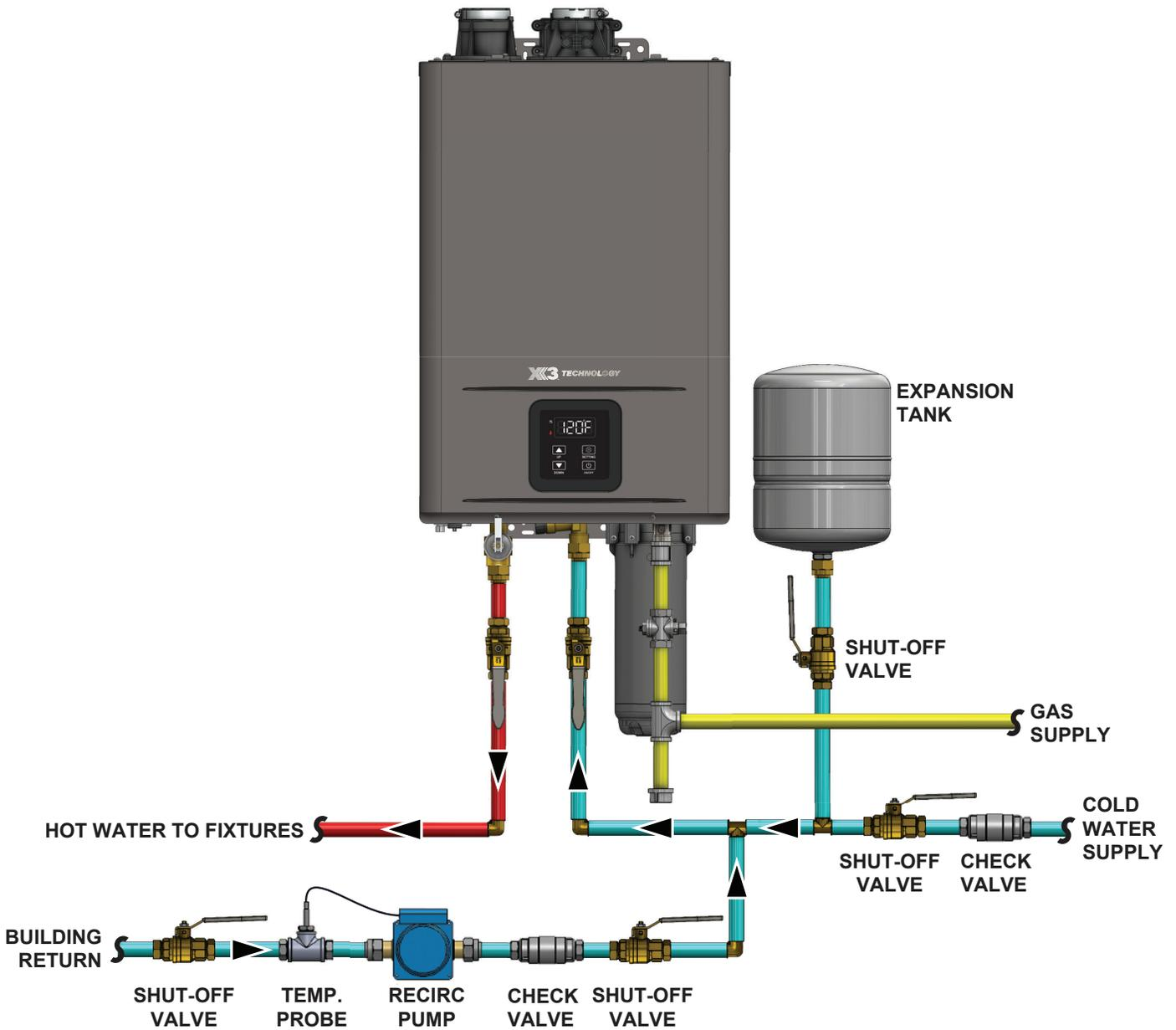
Figure 39 - Recommended Recirculation Diagram
