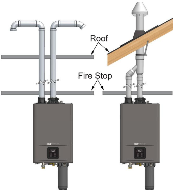
Figure 20 - Power Direct Vent Vertical Installation
