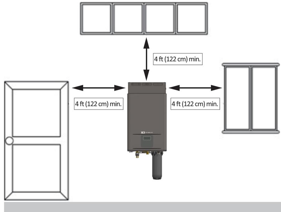
Figure 3 - Minimum Vent Clearances (Outdoor Venting)
