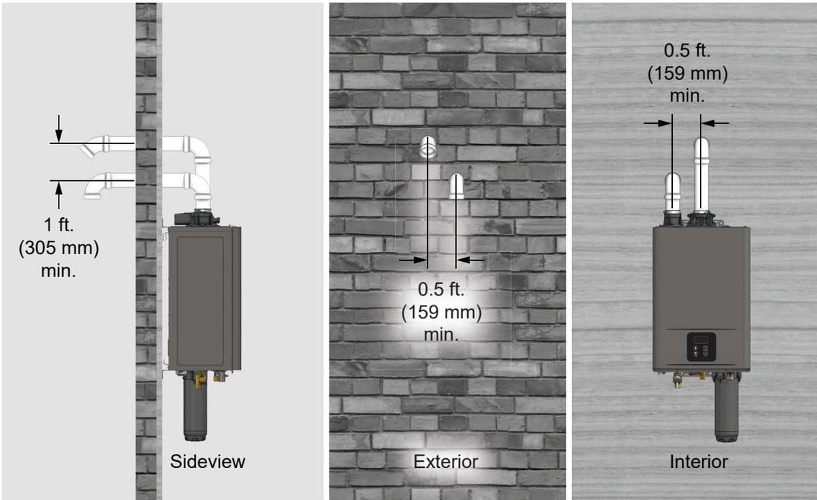
Figure 26 - Separate Sidewall Penetration Example A
