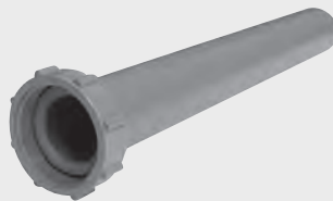
AW 1512PC CPVC 12" long sink tailpiece with nut and fluoroeastomer gasket.
