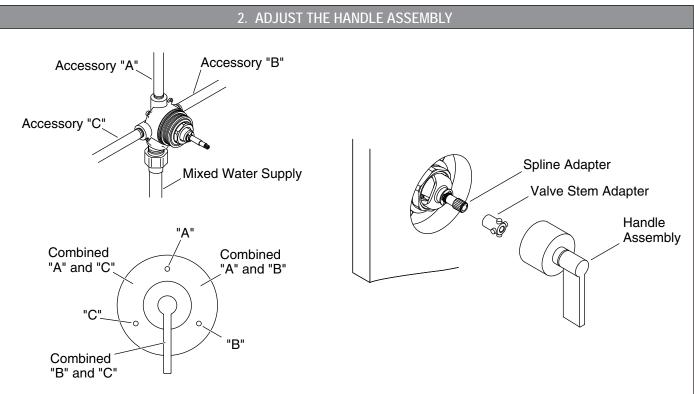
**NOTE:** Valve Operation. Water will flow from a single shower accessory when the control knob detent lines up with any of the large detents on the escutcheon. Water will flow from two accessories at the same time when the control knob detent is centered between two large detents on the escutcheon.
