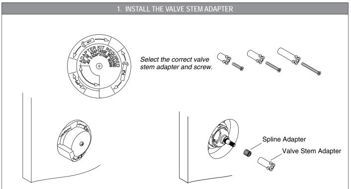
NOTE: Check the finished wall surface as related to the graphics on the plaster guard.
