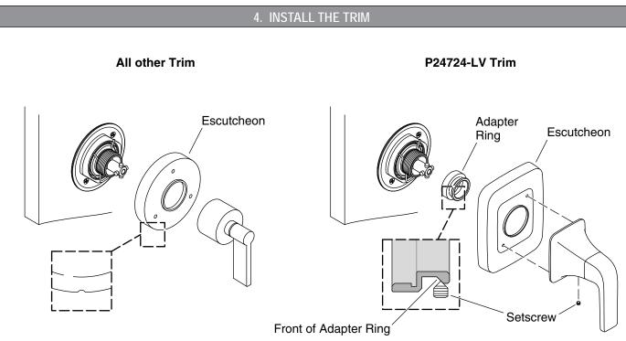
NOTE: If installing the P24724-LV trim, proceed to the "For P24724-LV" section below.
