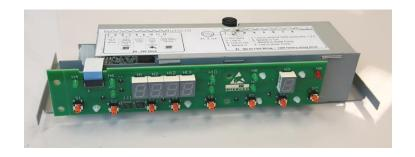
Figure 1: P-749B DC / HC Controller Replacement Kit
