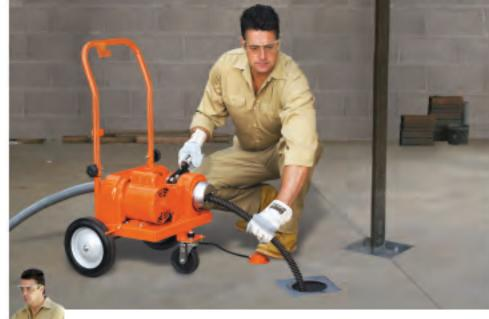
build-ups. For additional protection, the Rodrunner has an adjustable slip clutch, factory set at 18 - 20 ft. lbs.
